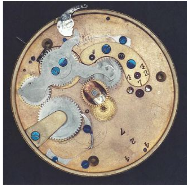
Figure 45. Early Full “Rocking Bar” SW M57 Movement
