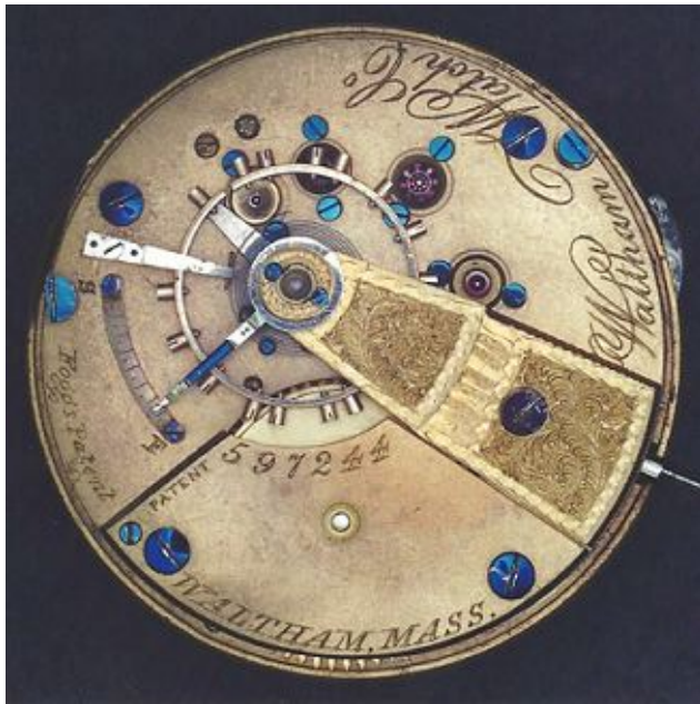
Figure 45. Early Full “Rocking Bar” SW M57 Movement
