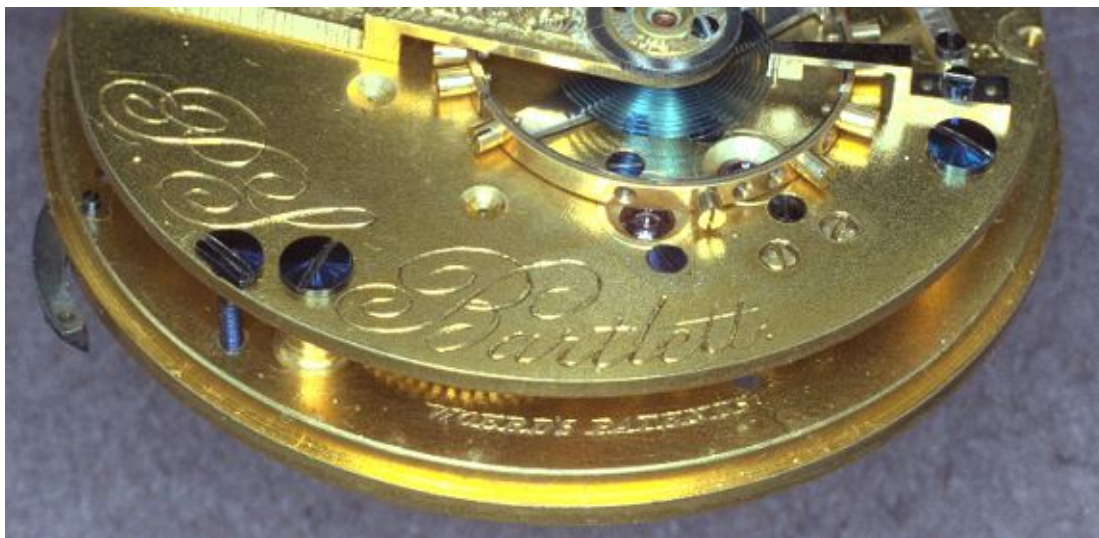
Figure 44. Inscription "Woerd's Patents" On Train Side of SW Pillar Plate, S/N 778362
