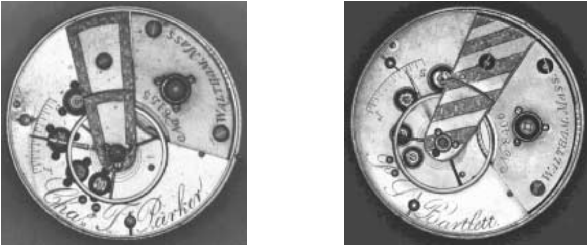
FIGURE 7. 15J Chas. T. Parker 8153 with real jewel settings and 11J P.S. Bartlett 8406 with burnished jewels
