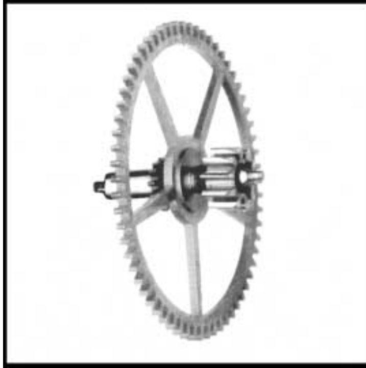
FIGURE 23. C.W. Fogg's patented safety center pinion (pinion unscrewed in picture)
