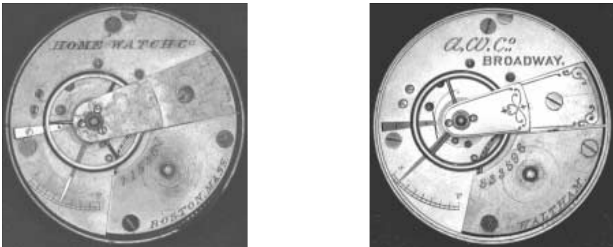
FIGURE 16. Example HWC and Broadway grade Model 57 7J Movements
