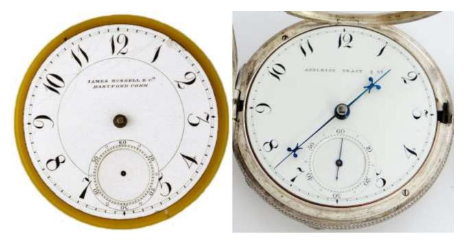
The fancy dial on the left is the dial on JR #20145 that was on the opening slide. The dial on the right is from Appleton Tracy #6716, made Dec 1858. Note the signature is in a straight line.
