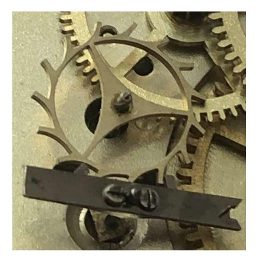
The picture is a little blurry, but not bad taken with my phone. I haven't used my digital camera for a long time. Note the blunt-end escape wheel. What I mean by "blunt-end" is the shaft of a tooth is squared off where the end of the tooth is the same size as the shaft. Also note the three spokes join the outer wheel at the base of the teeth. Here is picture of the actual factory part. [NS]
