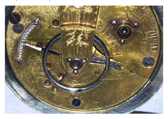
Note sprung under hairspring with hidden stud and applied index. The applied hairspring anchor is a repair. The style of the Dennison signature is consistent with a PSB, and although orientated correctly, the engraving on the barrel bridge is similar but still different from early AT movements.
